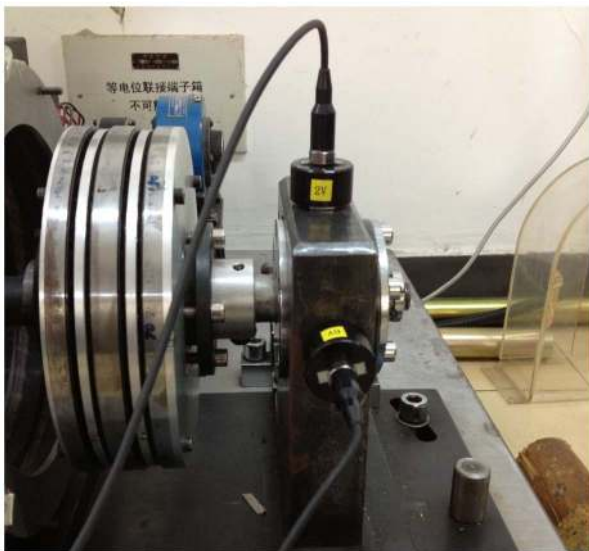
Figure 7. Install location of the acceleration sensor. doi:10.1371/journal.pone.0109166.g007
