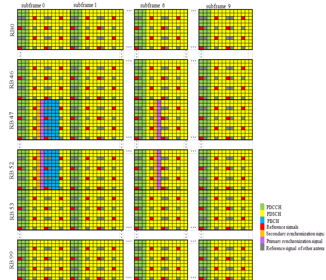
Figure 5.15 FDD Downlink physical layer configuration for 20 MHz system bandwidth and 4 antenna ports.
