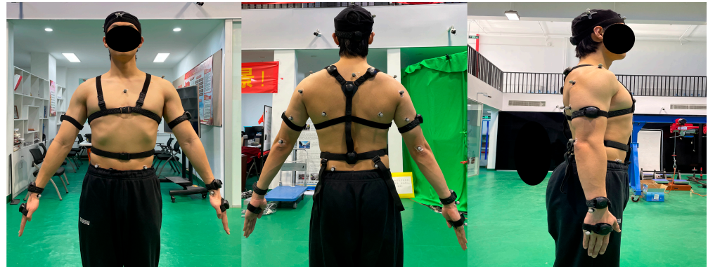
Figure 1. Placements of 11 IMUs and 25 reflective markers on a participant.
