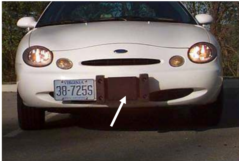
Figure 2.11. Front Radar Unit.
