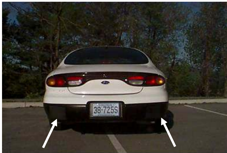
Figure 2.12. Rear Radar Units Embedded in Black Bumper.
