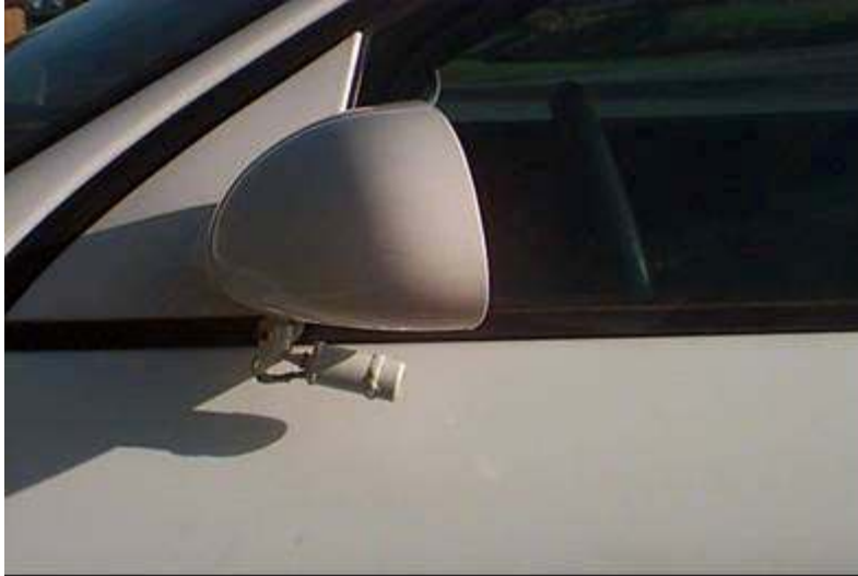
Figure 2.7. Camera Mounted Under the Side Mirror.
