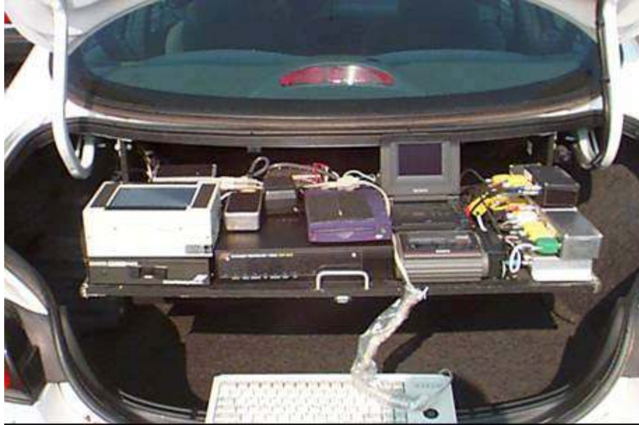
Figure 2.13. Data Collection Systems Storage Unit.
