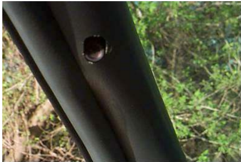
Figure 2.6. Driver's Face Camera Mounted in the A-pillar.
