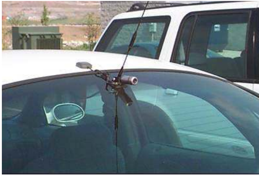
Figure 2.5. Rearview Video Camera above the Rear Window.
