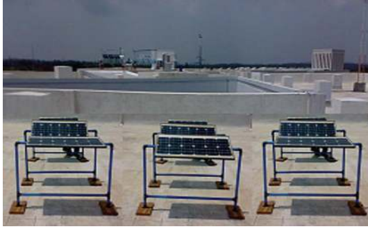
FIGURE 10: Practical setup of a 3 \times 3 array employing tilting modules for different shades.
