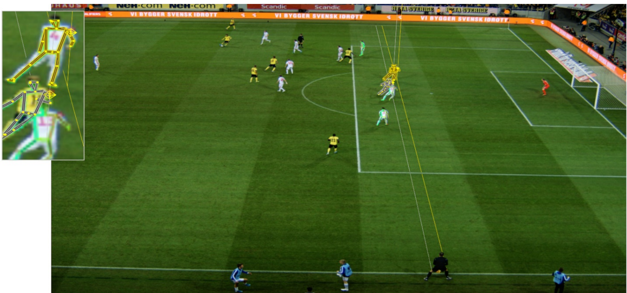
Figure 17. TRACAB Gen5 Technology for player tracking [294].
