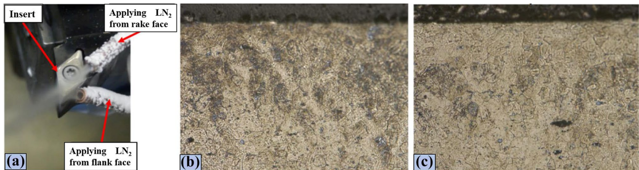
Fig. 19 a Cryo-turning; SEM micrograph of surface and sub-surface of the turned surface of NiTi alloy during b dry and c cryo-turning [139]
