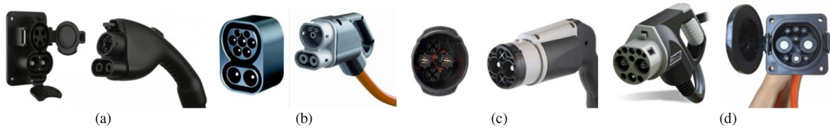
FIGURE 12. Plug for DC charging- (a) CCS/Combo for US, (b) European, (c) CHAdeMO, and (d) Chinese GB/T. Image courtesy: SAE and CHAdeMO.
