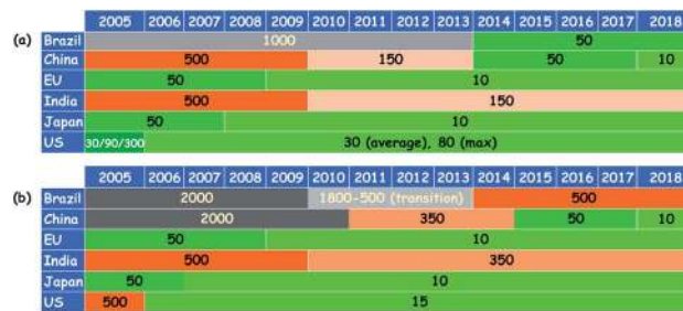
Fig. 1 The trend of stringent rules imposed on the sulfur level of motor liquid fuels over the years in different regions (a) gasoline and (b) diesel fuel). Adapted from ref. 3 with permission from The International Council on Clean Transportation.
