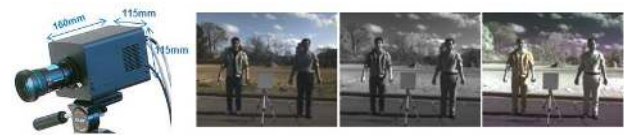
Fig.9. The Multiband Camera used in [203] and Sample Images (From Left to Right: Visible Band, 740nm Band, Three NIR Bands)
