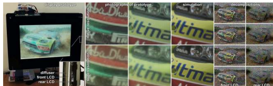
Fig. 1. Compressive superresolution display. The proposed display architecture comprises two stacked high-speed liquid crystal displays (LCDs) covered by a diffuser (left). A target high-resolution image is then decomposed into a set of patterns that are shown on the front and rear LCD in quick succession (right). Compared to the native resolution of each panel (center, top row), the proposed compressive display approach achieves significant improvements in resolution (center, bottom row) without any mechanically moving parts.
