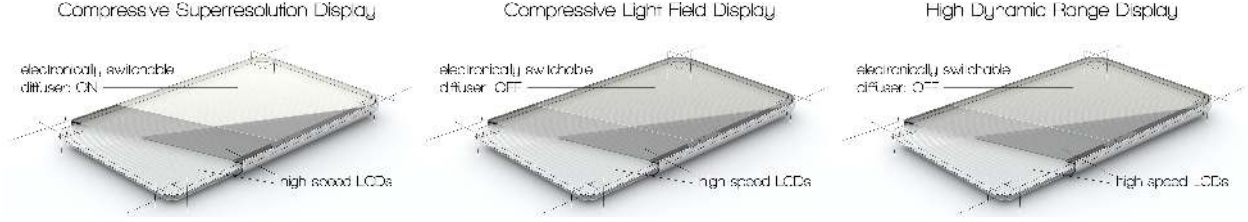
Fig. 2. Conceptual sketch of a multi-purpose compressive display. The device consists of two high-speed liquid crystal panels covered with an electronically-switchable diffuser. With the diffuser being activated, the display is capable of showing superresolved 2D images (left). The diffuser can be deactivated and becomes transparent. In this configuration, the device can emit either a light field for glasses-free 3D display (center) or a high dynamic range image (right).
