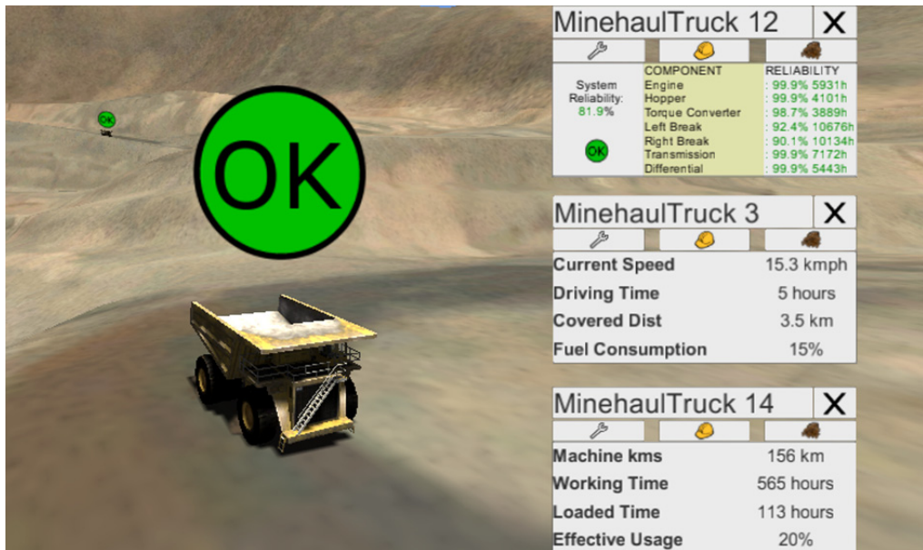
Fig. 7. Operational and reliability information of the mining truck. Colors are related to the reliability condition of the equipment part
