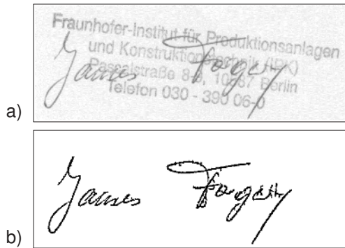
Fig. 14. Removal of stamps and other imprints: (a) original signature image with overlapping stamp (b) signature image after stamp removal
