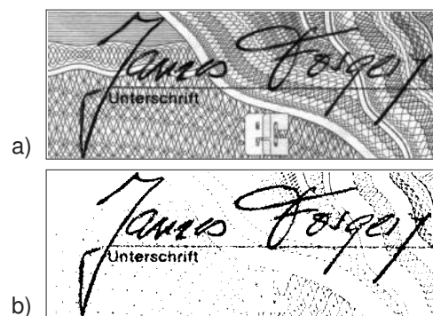
Fig. 1. Poor separation of handwriting from textured background: (a) original signature image, (b) signature image after processing
