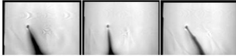
FIGURE 11. MR images of 3 different concentric tube robot needle insertion trajectories to the same target location in the soft gelatin phantom. Closed-loop inverse kinematics was utilized to reach the same target with different joint space configurations.
