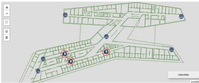
Fig. 10. An example of localization of three points (red circles) in the simulated environment, with six different 5G antenna placements. This simulation component is tested via a simple user interface that allows the placement of 5G antennas anywhere on the vectorized GeoJSON version of the 2D floor plan (generated from the as-is BIM representation).
