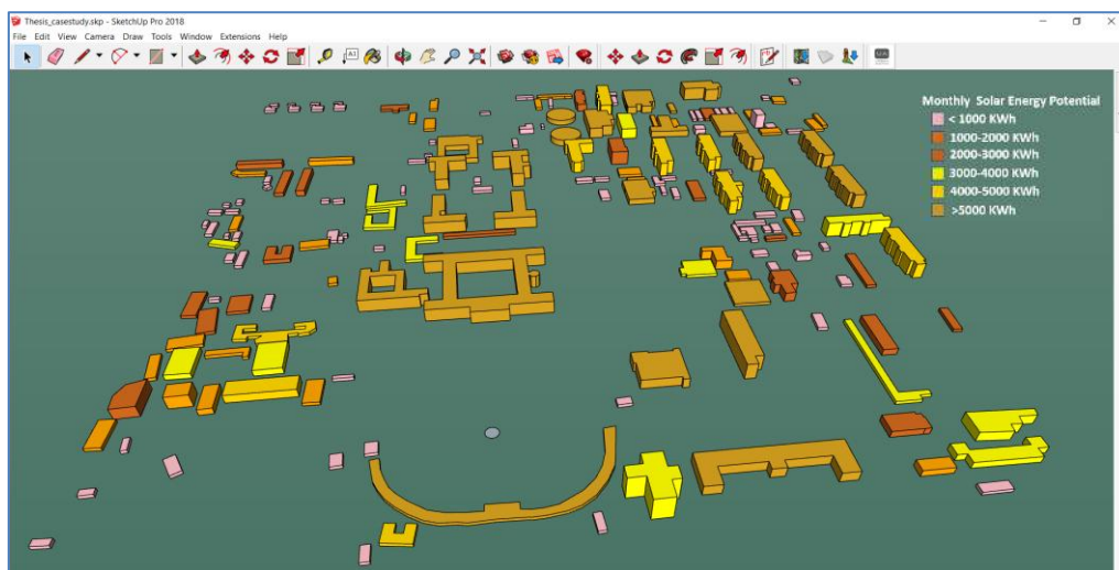
Fig-16: Visualization of Solar Energy Potential at city level which is predicted by AI
