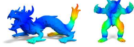
Figure 4: Absolute values of the 4 th eigenfunction of the Laplace-Beltrami operator of the dragon model (left) and of the 8 th eigenfunction of the armadillo model (right), both corresponding to non-repeating eigenvalues. The absolute values of these functions increase as the color changes from blue to red. Note that these values are not preserved under the bilateral symmetries.
