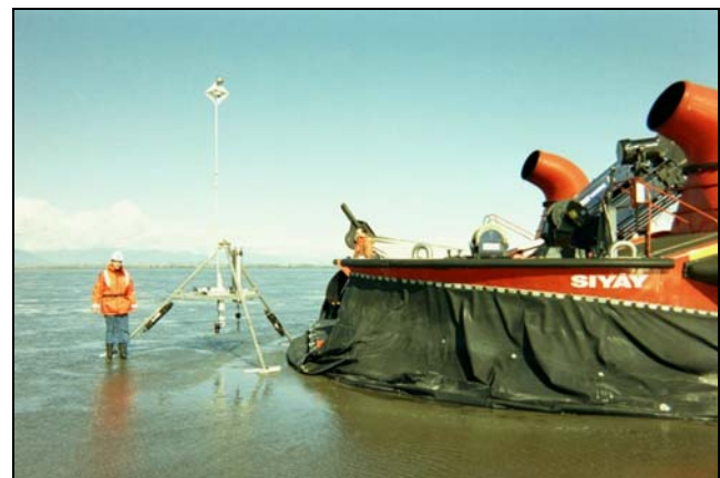
Fig. 4. Deployment of Norton on Roberts Bank March 23, 2003 using the Canadian Coast Guard Hovercraft Sivay . A radar reflector and flashing light were mounted on a pole above the tripod.
