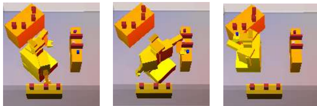
Fig. 5: Plan to pick an object from an awkward location on one table, and move it to the back table.
