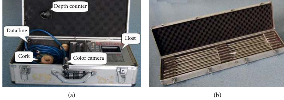
FIGURE 9: YTJ20 borehole detection recorder. (a) Detection recorder host. (b) Guide rod.
