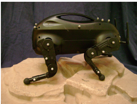
Fig. 1. The BDI LittleDog robot. Each leg has three actuated degrees of freedom, two at the hip ( \theta_{hip,x} , \theta_{hip,y} ), and the knee joint \theta_{knee} . The whole system therefore has 18 degrees of freedom, three per leg plus ( x,y,z,roll,pitch,yaw ) of the body.
