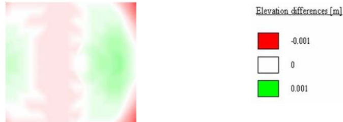
FIG. 3. Elevation differences, k_l changed by +20% (convergent case)
