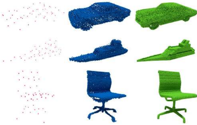
Figure 6: Qualitative results for our point cloud upsampling. Severely under-sampled input point clouds (50 points) are shown in red. The network predictions and ground truth point clouds are shown in blue and green respectively (16000 points).
