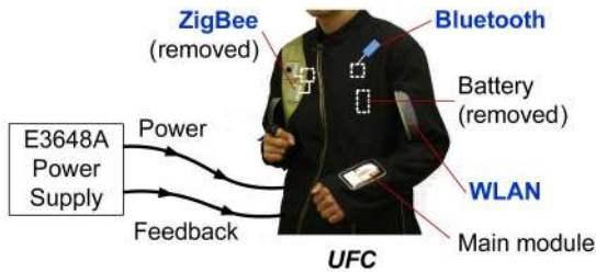
Fig. 5. Appearance of UFC. A power supply is directly connected for experiments.
