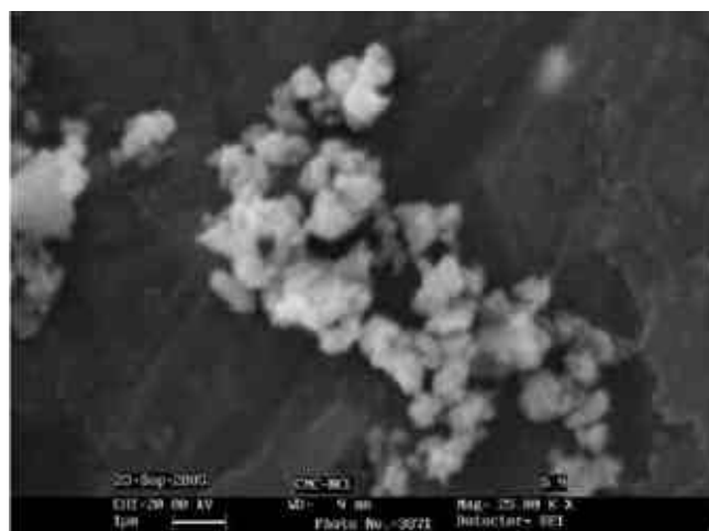
Figure 4. SEM of NT powder calcined at 700°C.
