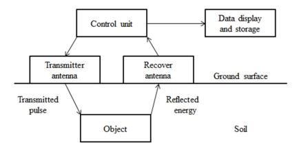
Figure 1. Components of a typical GPR system.
