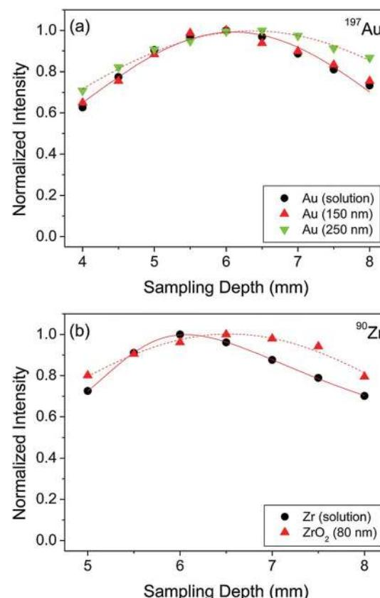
Fig. 3 Sampling depth profiles of (a) Au and (b) Zr in the form of aqueous solution with a concentration of  $10 \mu\text{g L}^{-1}$  and discrete NPs. Reproduced from Ho *et al.*<sup>38</sup> with permission from the Royal Society of Chemistry.
