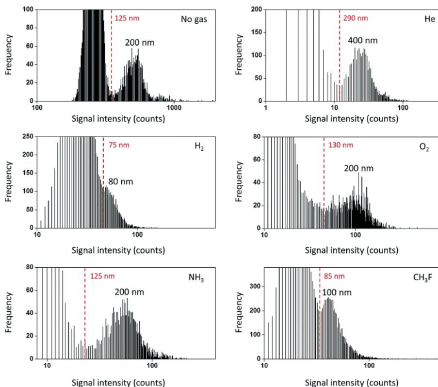
**Fig. 4** Frequency distribution for the lowest NP sizes detectable using different reaction gases in ICP-TQ-MS for  $\text{SiO}_2$  particle analysis. Practical  $\text{LODs}_{\text{size}}$  are indicated in red in each figure. Frequency refers to the number of events of each type (background or NPs) detected. Reproduced from Bolea-Fernandez *et al.*<sup>56</sup> with permission from the Royal Society of Chemistry.
