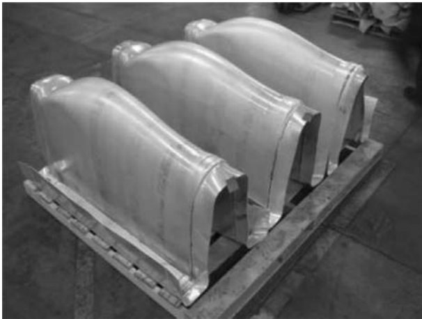
Figure 25. Non-planar clamp line SPF forming [43].
