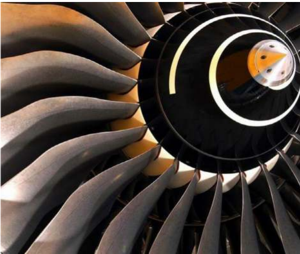
Figure 28. The titanium fan blade for Trent 900 engine.
