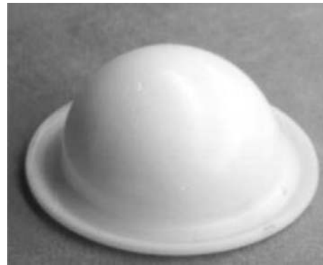
Figure 30. First bubbles superplastically formed from ceramic sheet.
