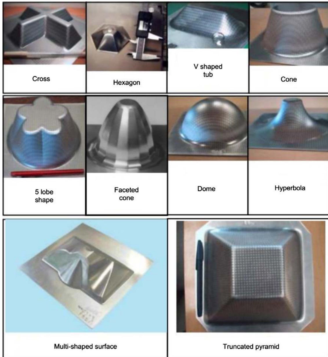
Figure 36. Shapes used to demonstrate the ability of the process and for experiments [60].
