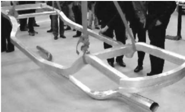
Figure 9. An aluminum lower rail for the Volvo car (AP&T, Sweden) [23].
