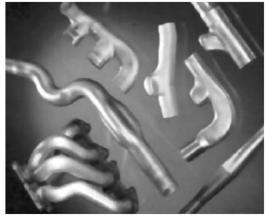
Figure 7. Exhaust parts produced by hydroforming (Schuler Hydroforming, Germany) [23].
