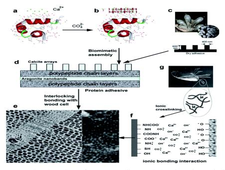
**Figure 5.** (**a**,**b**,**d**) Synthesis of soy protein adhesives, (**c**,**g**) gecko and mussel adhesive proteins, (**e**,**f**) mechanical and ionic crosslinking mechanisms at the surface, Reproduced from [211], Royal Society of Chemistry, 2017.
