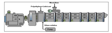
Figure 2. Extruder machine for WPC manufacturing.
