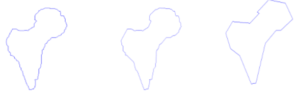
Fig. 8 A silhouette shown in various evolutionary stages. From left to right the polygons contain 379, 50 and 15 vertices respectively.
