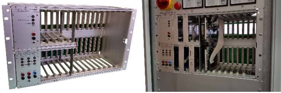
Fig. 3: Left: An empty subrack (19" / 6U) of the DSP-System. The backplane and the two power-supply units (5V, 15V, 24V) can be seen. Right: A partially populated subrack, already built into a control cabinet.
