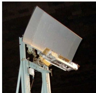
Figure 14. Photo of the antenna prototype installed on an anechoic chamber tower.
