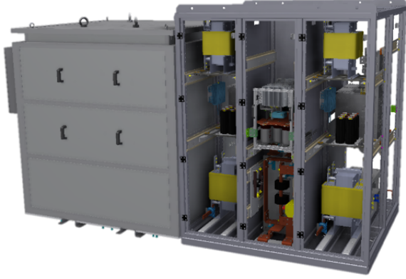
Fig. 3. SATURN power converter used for various applications at CERN.
