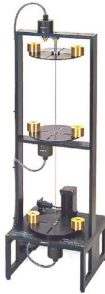
Figure 4.14 – Torsional apparatus (ECP model 205a) used for the experimental analysis. The three disks are comprised of block masses which can be added or removed to alter the inertia of each disk (and thus alter the dynamics of the system). Each disk is vertically suspended on a spring with a variable spring constant. The actuator is located on the bottom of the device.
