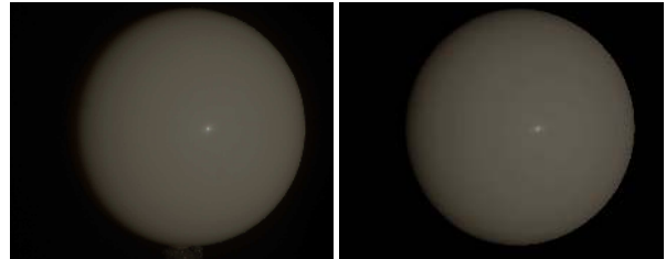
Figure 4: Two log images of a sphere (alumina oxide). A real image is shown on the left. A synthesized image using tabulated BRDF data is shown on the right.
