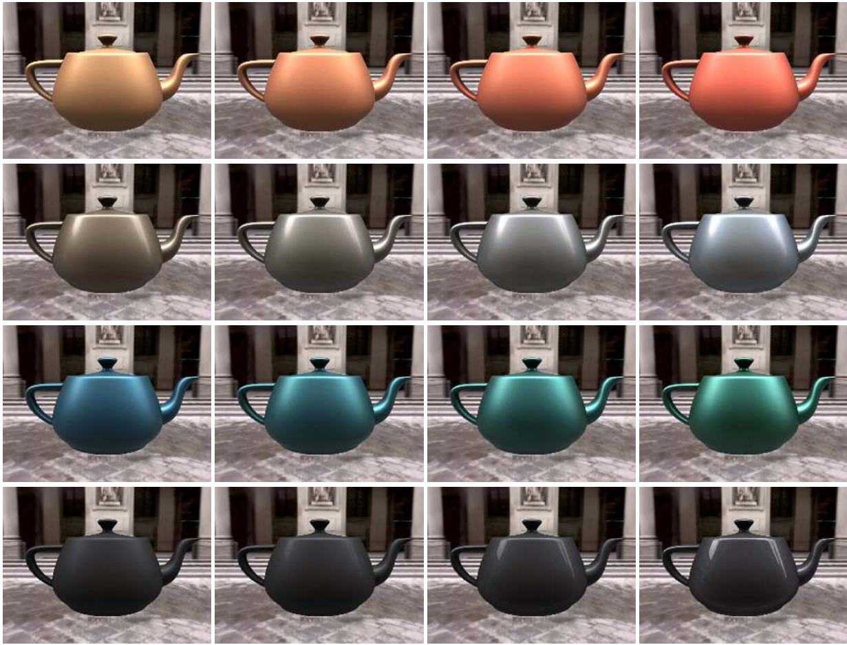
Figure 15: Navigation in the linear space. Each row corresponds to changing one parameter of the model. The first row shows an increase in the redness trait applied to the GoldPaint BRDF. The second row illustrates an increase in the silverness trait applied to the SpecularGold BRDF. Row three applies the gold-like trait to the BlueGlossyPaint BRDF. The fourth row shows an increase in the specularness trait applied to the BlackMattePlastic BRDF.
