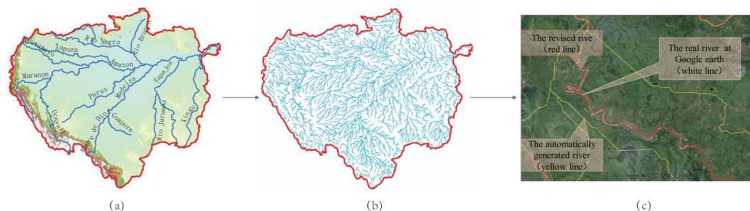
Fig. 2 The process of revising DEM and determining the location of correct river (e.g. Amazon river Basin). (a) The original SRTM-DEM. (b) The river obtained after modifying the DEM, based on the digital rivers drawn according to the real river in Google earth. (c) The comparison of the rivers before and after DEM modified.
