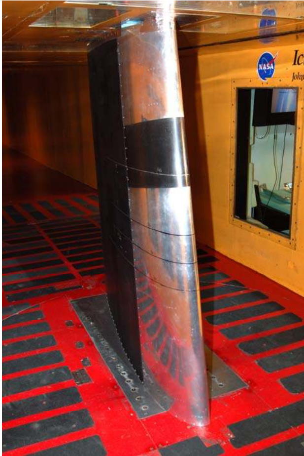
Figure A5. Entry F Business Jet Wing (a = left) Suction Side, (b = right) Pressure Side. Note: a portion of the aluminum leading edge was painted black for an earlier test.
