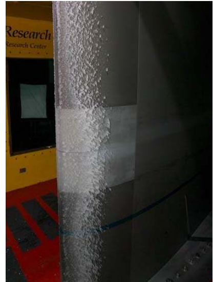
Figure B6. Case C-1999 ice accretion (a = top left) pressure side, (b = top center) leading edge, (c = top right) suction side, (d = middle left) pressure long shot, (e = middle center) tracing of C-1999 and C-1999m, (f = middle right) pressure long shot. (g = bottom left) Case C-1999m pressure long shot, (h = bottom right) C-1999m suction long shot.
