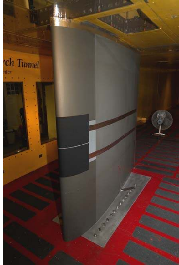
Figure A2. Entry C: NACA 23012 airfoil in IRT (a = left) Pressure Side, (b = right) Suction Side.
