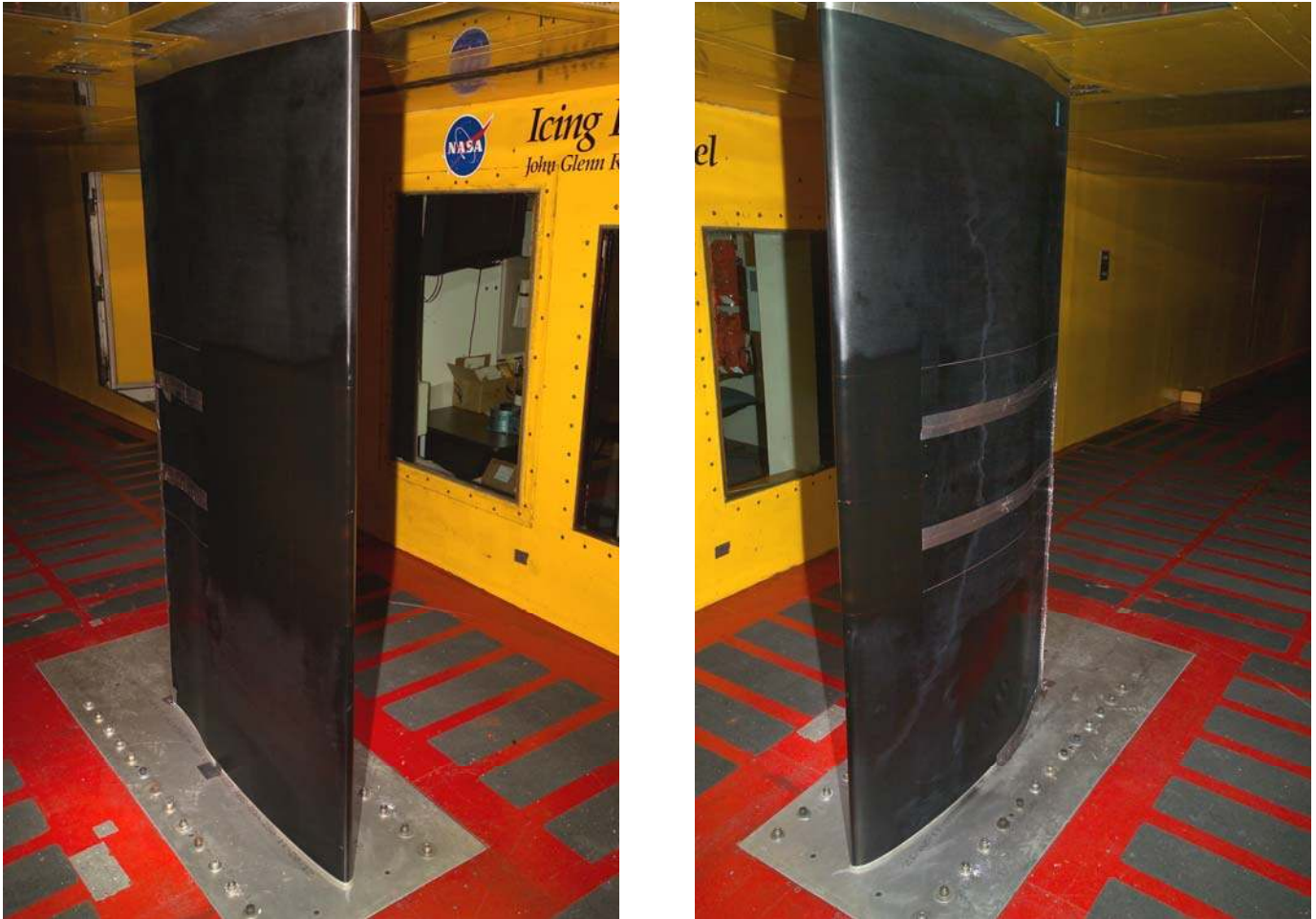
Figure A1. Entry B NLF 0414 airfoil in IRT (a = left) Pressure Side, (b = right) Suction Side.
