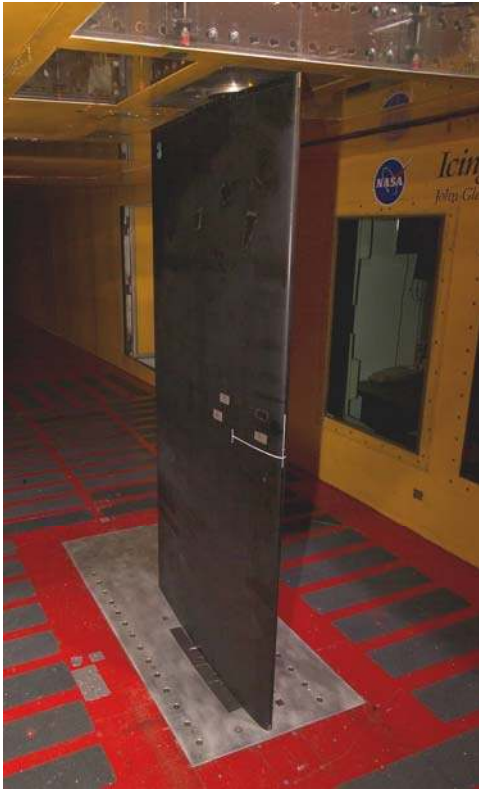
Figure A4. Entry E Commercial Tail airfoil in IRT (a = left) Pressure Side, (b = right) Suction Side.
