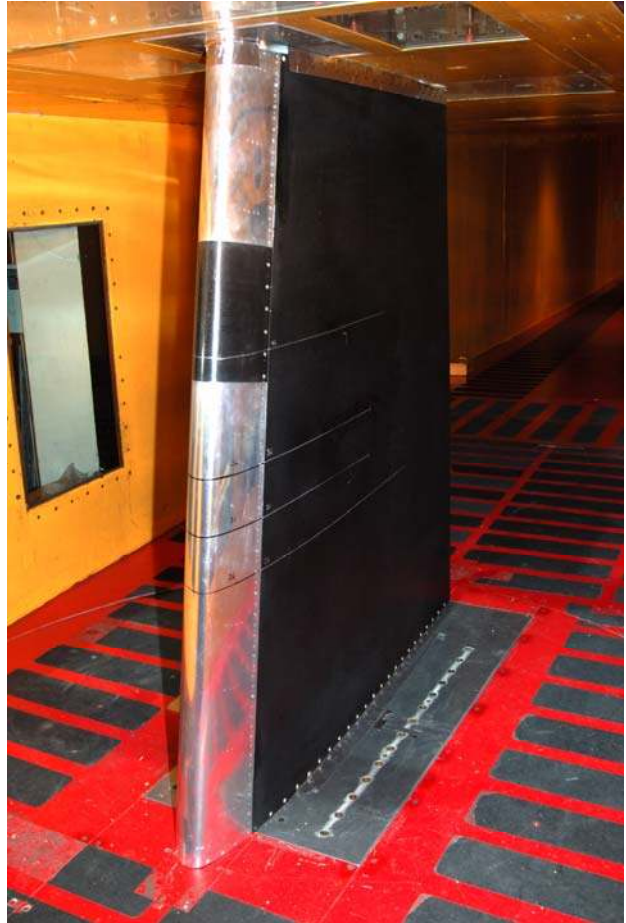
Figure A5. Entry F Business Jet Wing (a = left) Suction Side, (b = right) Pressure Side. Note: a portion of the aluminum leading edge was painted black for an earlier test.
