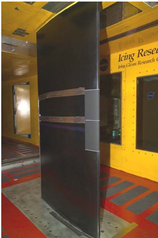
Figure A3. Entry D (and A) GLC 305 (a = left) Suction Side, (b = right) Pressure Side.
