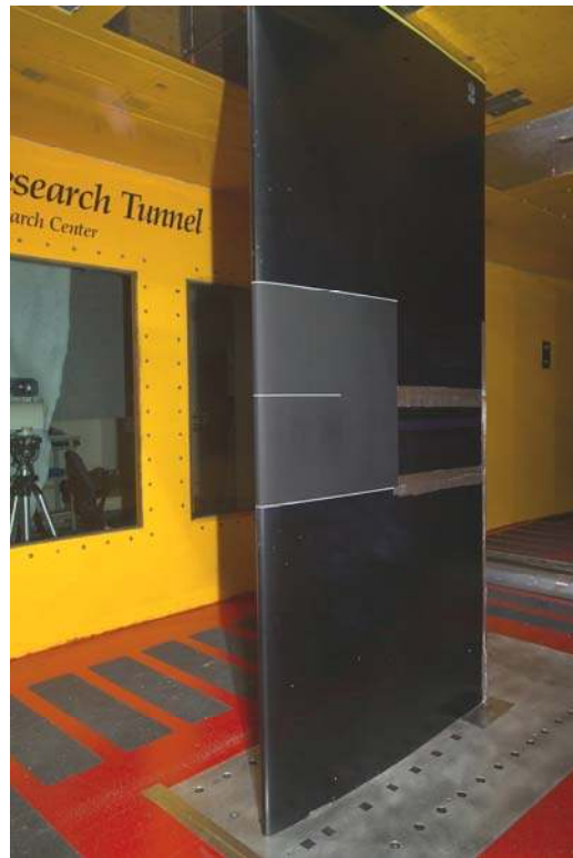
Figure A3. Entry D (and A) GLC 305 (a = left) Suction Side, (b = right) Pressure Side.
