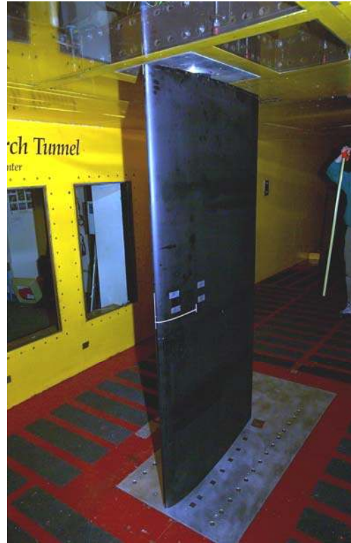
Figure A4. Entry E Commercial Tail airfoil in IRT (a = left) Pressure Side, (b = right) Suction Side.
