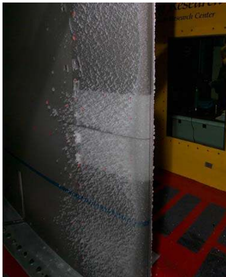
Figure B6. Case C-1999 ice accretion (a = top left) pressure side, (b = top center) leading edge, (c = top right) suction side, (d = middle left) pressure long shot, (e = middle center) tracing of C-1999 and C-1999m, (f = middle right) pressure long shot. (g = bottom left) Case C-1999m pressure long shot, (h = bottom right) C-1999m suction long shot.
