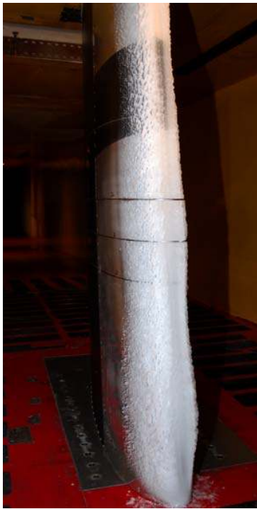
Figure B5. Case F-7575r4 ice accretion (a = top left) suction side, (b = top center) leading edge, (c = top right) pressure side, (d = bottom left) suction long shot, (e = bottom center) tracing, (f = bottom right) pressure long shot.
