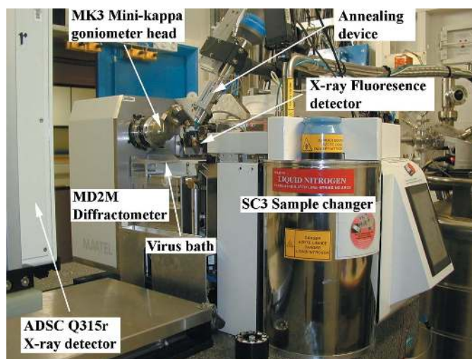
Figure 7 Photograph of the routine sample environment set-up in the ID14-4 experimental hutch.
