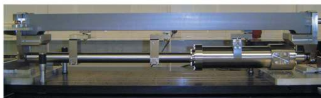
Figure 6 (a) Technical drawing of the toroidal mirror as mounted on ID14-4. The arrows indicate how the mirror is rigidly attached to the granite table. (b) A picture of the ID14-4 toroidal mirror taken in the metrology laboratory of the ESRF (courtesy of A. Rommeveaux, ESRF Metrology Group).
