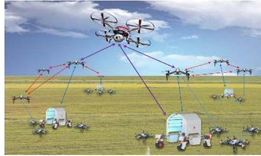
Fig. 1. Scenario of a smart agriculture farm that is facilitated with a proper coordination of (i) a team of aerial drones to survey the fields and to map weeds, yield and soil variation and (ii) a fleet of ground vehicles (specialized robots which consistently communicate with the survey drones) used for automated weeding, fertilizing and harvesting.
