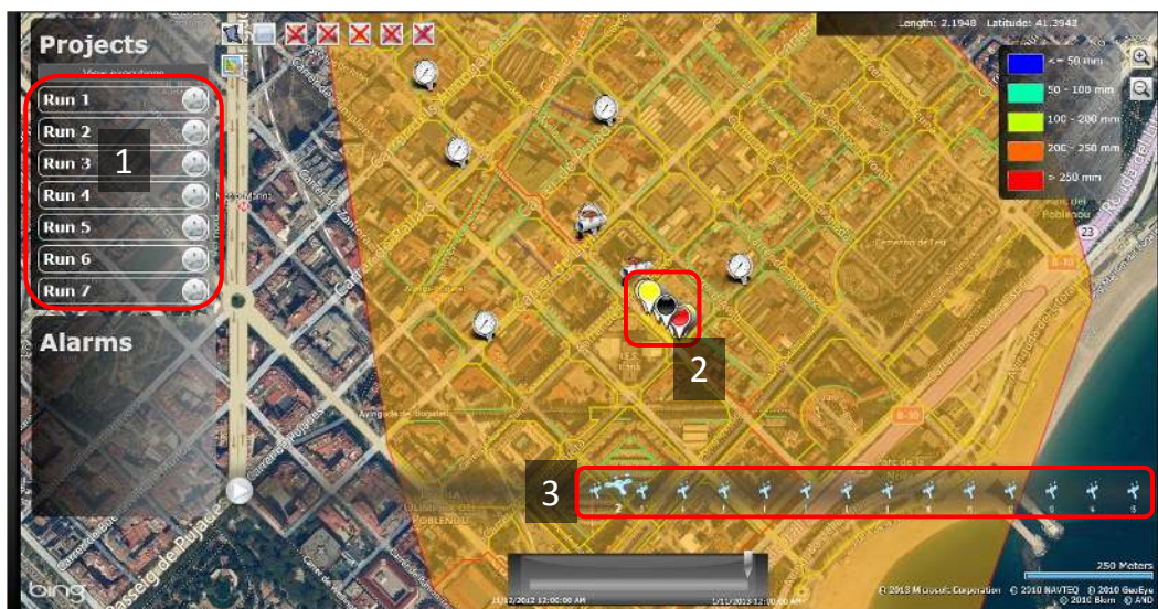
Figure 6 Example of the GIS viewer displaying the following layers : street layer, DMA network wrapping area (label ‘1’), DMA network pipes coloured according to their diameter, DMA network sensors distinguishing between the inner pressure sensors (label ‘2’) and the pressure / flow sensors of the DMA inlets (label ‘3’).
