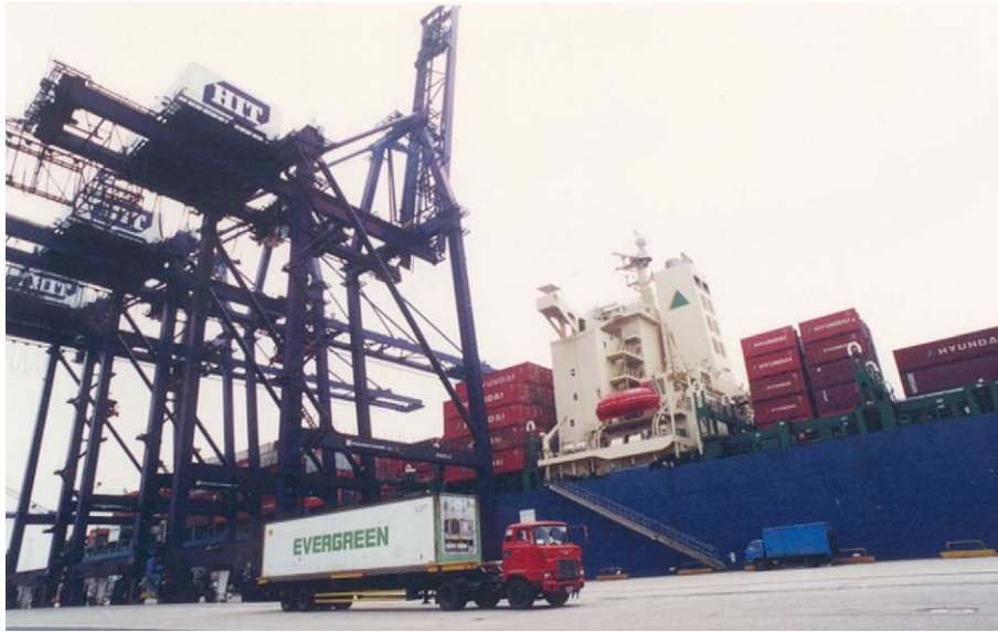
Fig. 3. Three QCs serving a vessel docked on the berth. An IT can also be seen. The QCs unload containers from the vessel and place them on ITs, which take them to the storage yard for storage until they are picked up by consignees. ITs also bring outbound containers from the storage yard for the QCs to load onto the vessel.
