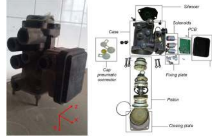
Fig. 1. EBS-5, TCM (left) and its sub-components (right).
