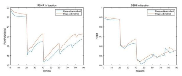
**Figure 3.** Levin image restoration experiment. Left is PSNR and right is SSIM. This paper used the same parameters and solution methods to test the performance of the two regular terms of WG-NGM and NGM under the same conditions.
