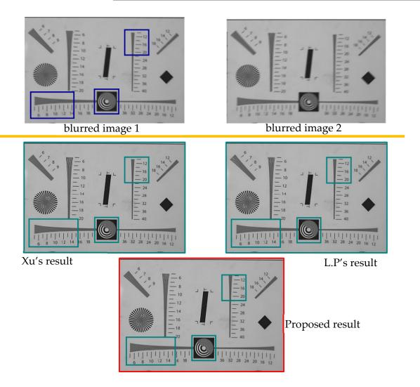
**Figure 10.** The input blurred images and the restoration. The top line is the blurred images 1 and 2; The middle line is the results of Xu's and L.P's methods as space-invariant. The bottom line is the deblurred image using the proposed method as space-variant.
