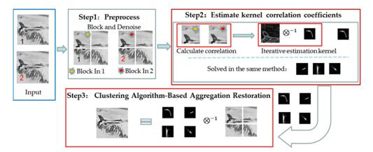
**Figure 1.** Structure flow chart: This figure describes the flow and components of the proposed algorithm. The input is two blurred images with different blurring patterns, but with the same object. The first step is pre-processing, which focuses on block splitting and de-noising. The second part estimates the blur kernel, block by block. The third step is the classification of the blur kernels using a clustering algorithm and the final restoration.
