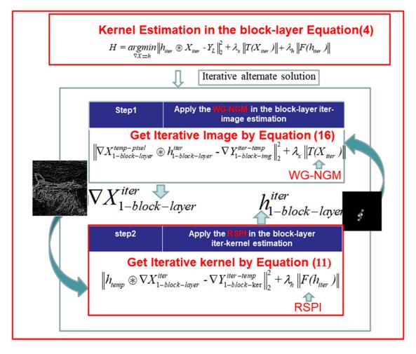
**Figure 2.** The block layer kernel estimation flow chart. According to the EM algorithm idea, iterative kernels are estimated alternatively with the iterative image, which needs to be fixed in the iterative image when estimating the kernel and vice versa.
