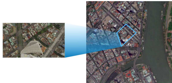
Figure 1: A figure showing the registration of two images from different domains. Left: an image from a UAV, Right: a satellite image.
