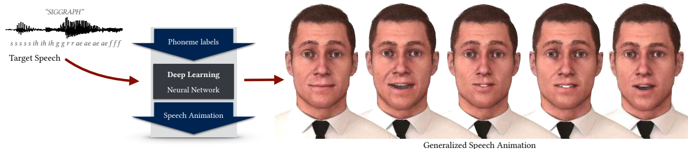
Fig. 1. A machine learning approach is used to learn a regression function mapping phoneme labels to speech animation. Our approach generates continuous, natural-looking speech animation for a reference face parameterization that can be retargeted to the face of any computer generated character.
