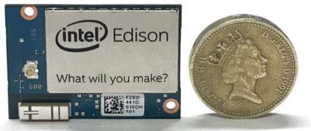
Fig. 6. Intel Edison features a dual-core Intel Atom CPU at 500 MHz, wireless connectivity, and compact physical dimensions at 35.5 \times 25.0 \times 3.9 mm. It is a small but powerful platform that is well suited for wearable devices.
