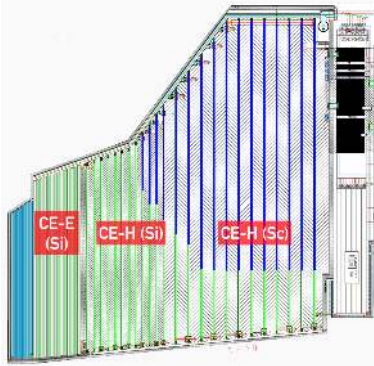
Figure 1. Scheme of the HGCAL subdetector used for this study [1] (not the last design version). Three main kinds of sensors distributed on layers are shown here: the electromagnetic section (CE-E-Si - 28 layers) and the two hadronic sections, one with silicon based sensors (CE-H-Si - 24 layers), the other with scintillator sensors (CE-H-Sc 16 layers).
