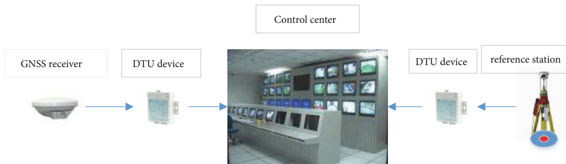
FIGURE 5: GNSS deformation monitoring system diagram consists of GNSS receiver, DTU, control center, and reference station.
