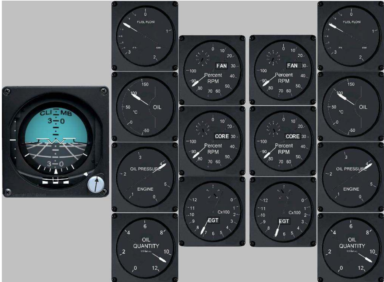
Figure 6.—Heads down instrumentation display showing variables for the two engines.
