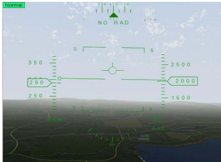
Figure 7.—Cockpit view with heads up display.
