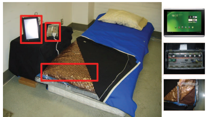
Figure 1. The pressure sensitive bedsheets consists of three parts: a textile sensor sheet, a sampling unit and a tablet.
